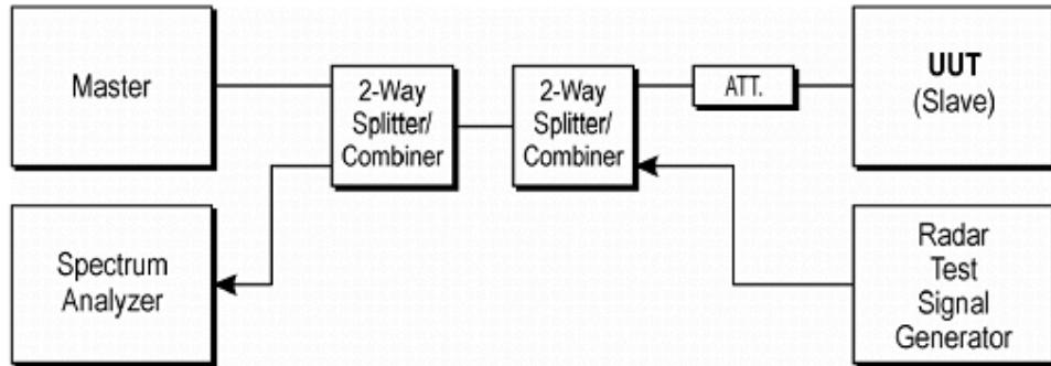
Figure 3-1. Conducted Test Setup for DFS
