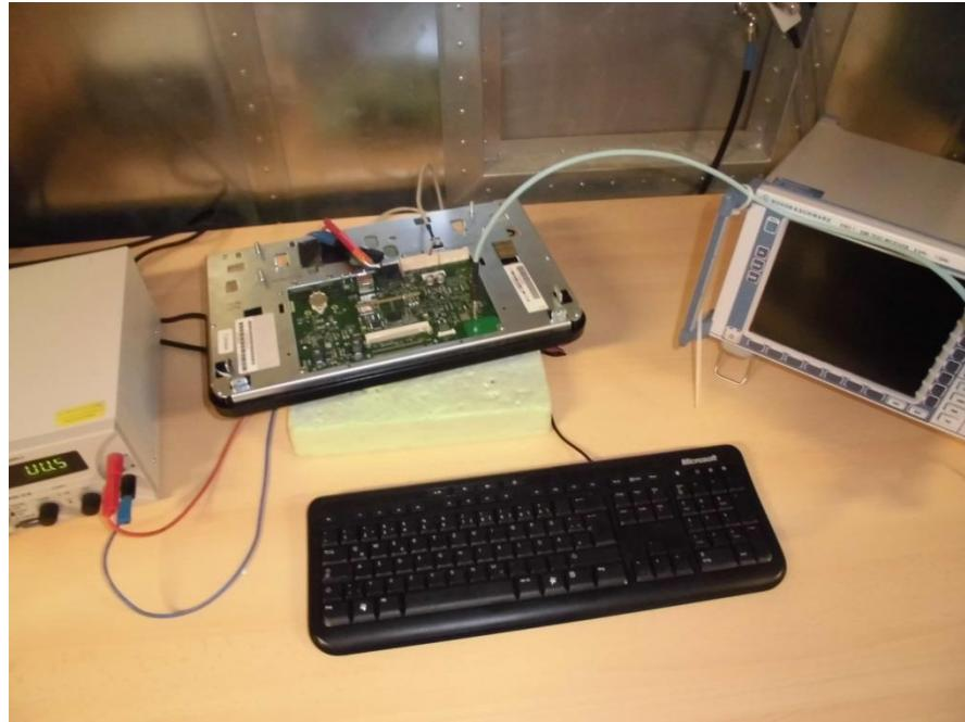
radiated disturbance 9kHz – 30MHz
