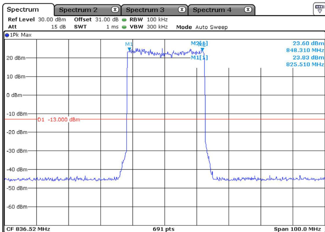
Downlink Band Pass – PCS 1900 mode DL
