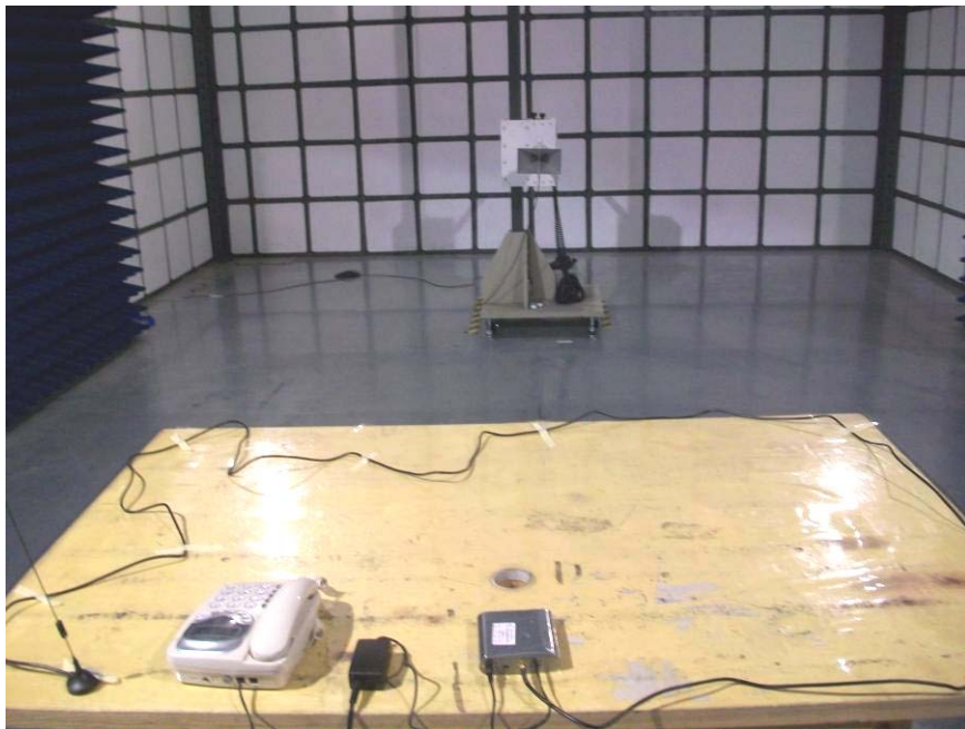
Radiated Emission Test View Above 1GHz
