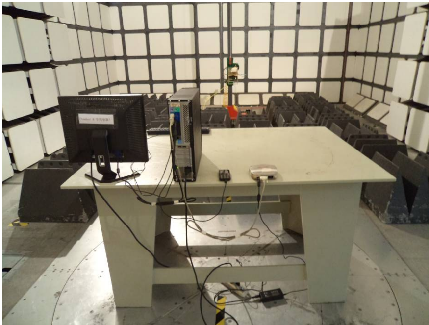
Radiated Emissions – Rear View (Above 1 GHz)
