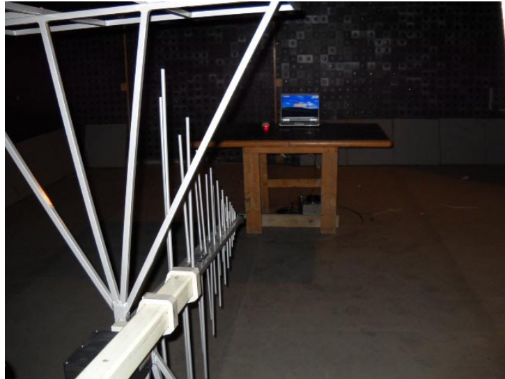
Photograph 7.2.1 Setup for radiated emission measurements in 30-1000 MHz
