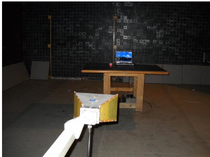
Photograph 7.2.2 Setup for radiated emission measurements above 1000 MHz
