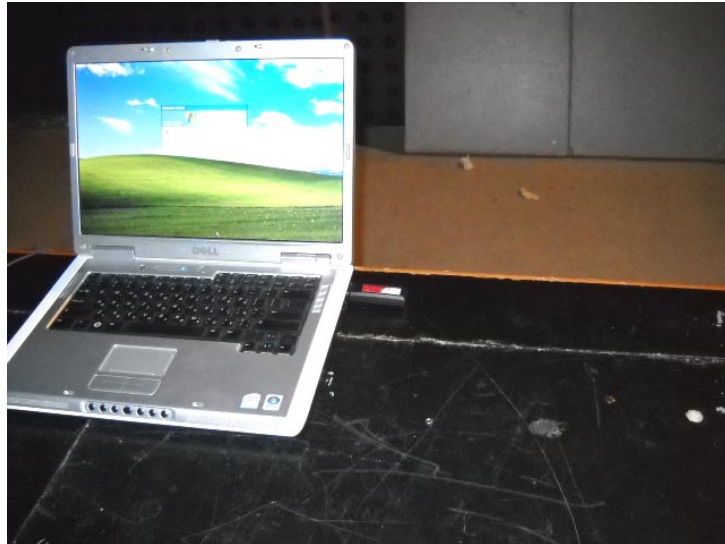
Photograph 7.2.3 Setup for radiated emission measurements, EUT close view
