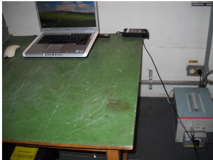
Photograph 7.1.1 Setup for conducted emission measurements
