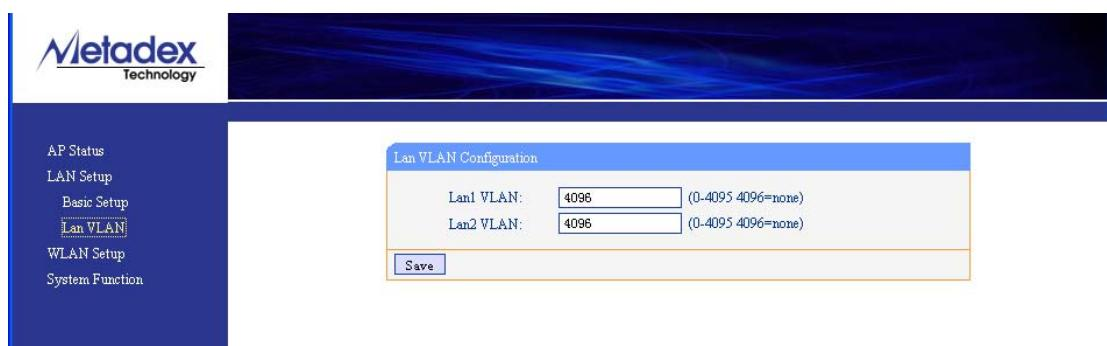
Set the VLAN number (0~4096 4096=none) of the LAN1 and LAN2 in LAN VLAN configuration.
