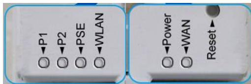
LED from left to right mean: LAN Ethernet Status 1, LAN Ethernet Status 2, PoE / PSE forwarding, WLAN Status; Power / Status, WAN Uplink / PoE. Provide “reset” button to resume to the factory default state in the event of an exception.
