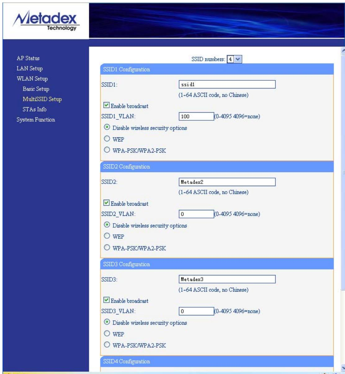
The screenshot shows the Metadex WLAN Setup interface. On the left, a sidebar lists navigation options: AP Status, LAN Setup, WLAN Setup, Basic Setup, MultiSSID Setup, STAs Info, and System Function. The main content area is titled "SSID numbers: 4" and contains four sections for configuring SSIDs:
