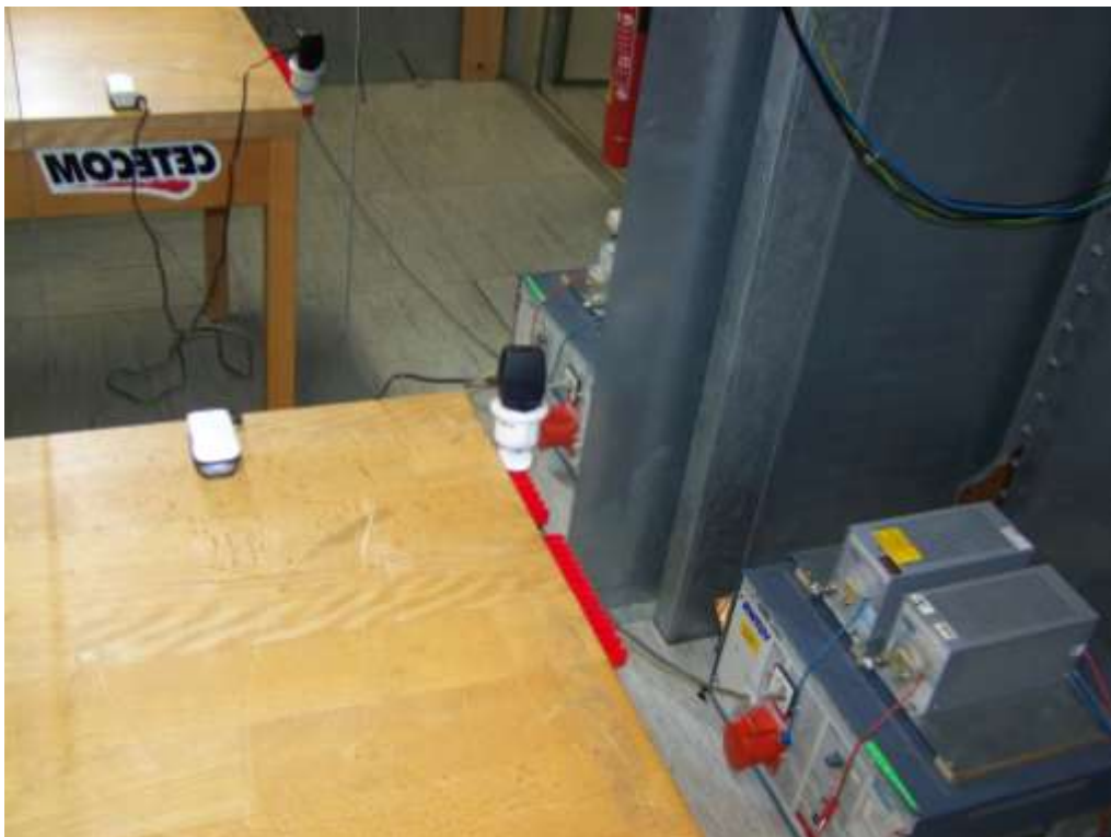
Photo: measurements of conducted emissions on AC-mains
