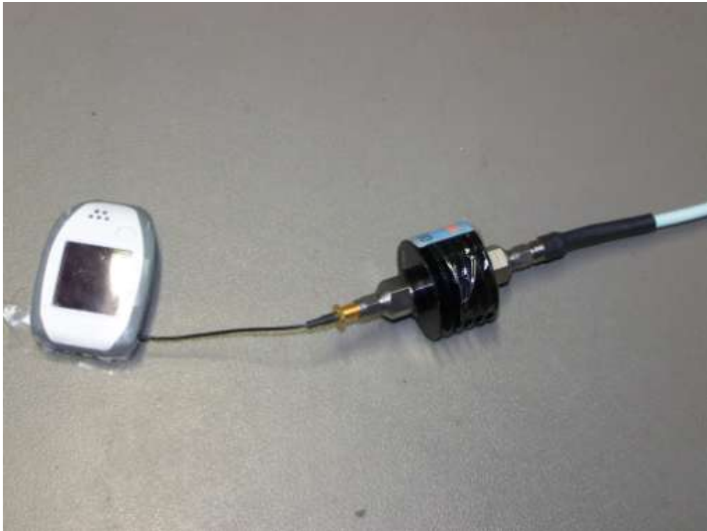
Photo: measurements of conducted rf-parameters
