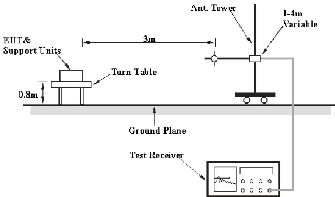
The radiated emission tests were performed in the 3 meters test site, using the setup accordance with the ANSI C63.17-2006. The specification used was the FCC §15.319(g).
