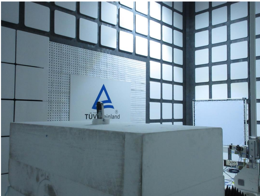
Photograph 6: Set-up for Spurious Emissions (Back View 4)
