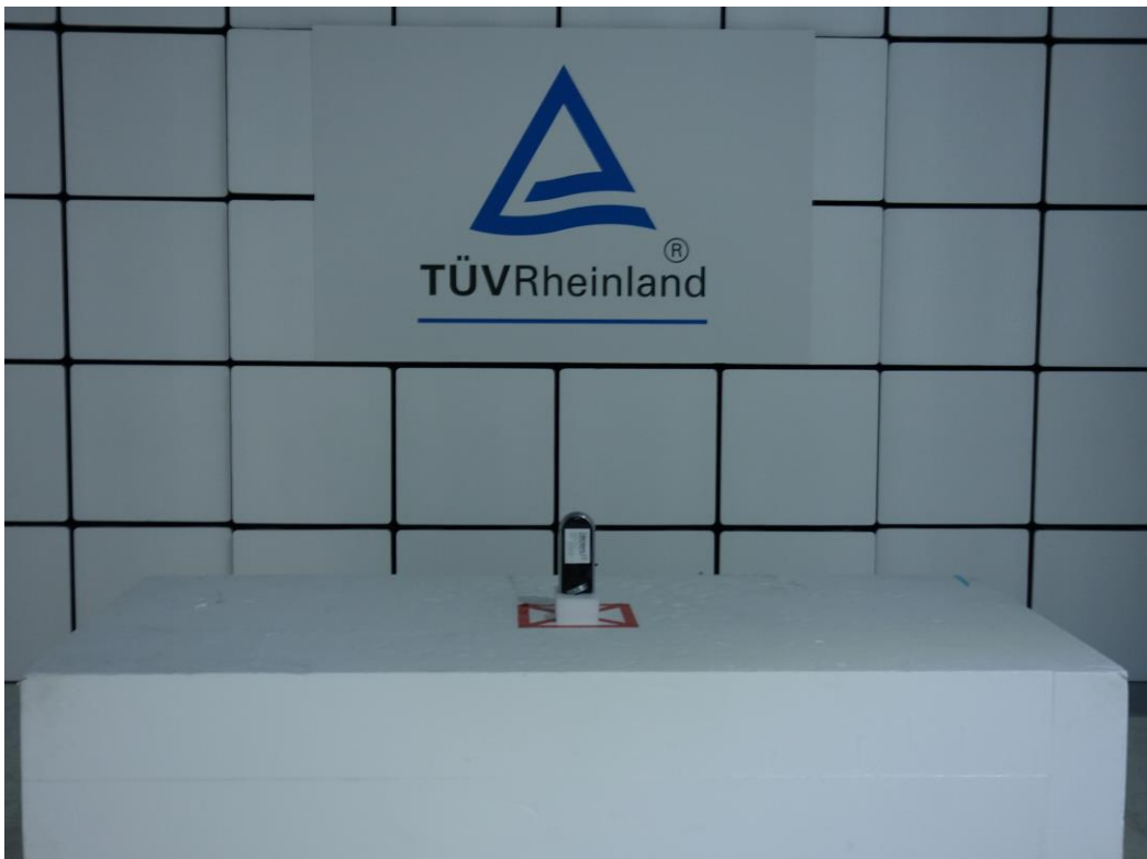
Photograph 2: Set-up for Spurious Emissions (Front View)
