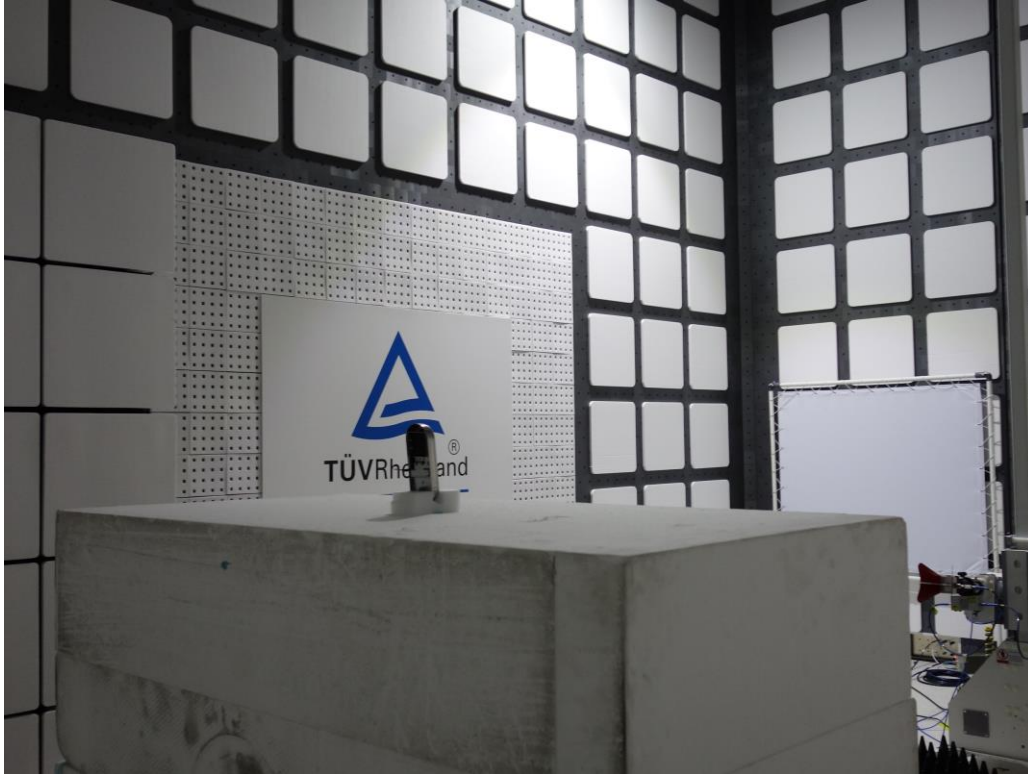
Photograph 3: Set-up for Spurious Emissions (Back View 1)
