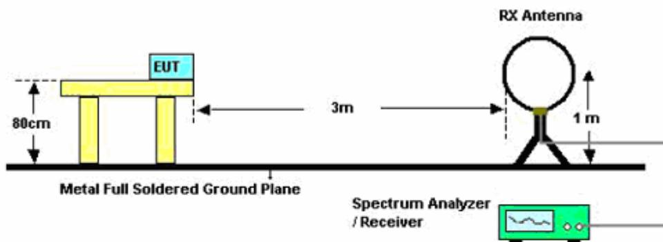
For radiated emissions 30MHz to 1GHz
