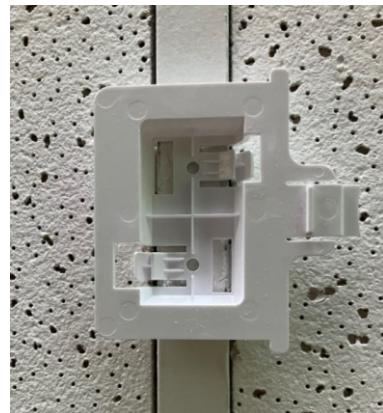
Plug in the network cable or other port cables and slide the unit onto the ceiling bracket until the latch clicks in place.
