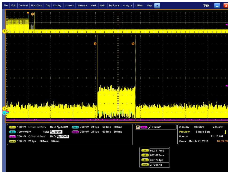
Figure 7: Master broadcasts five beacons (0.36ms) that include an 802.11h channel switch announcement.
