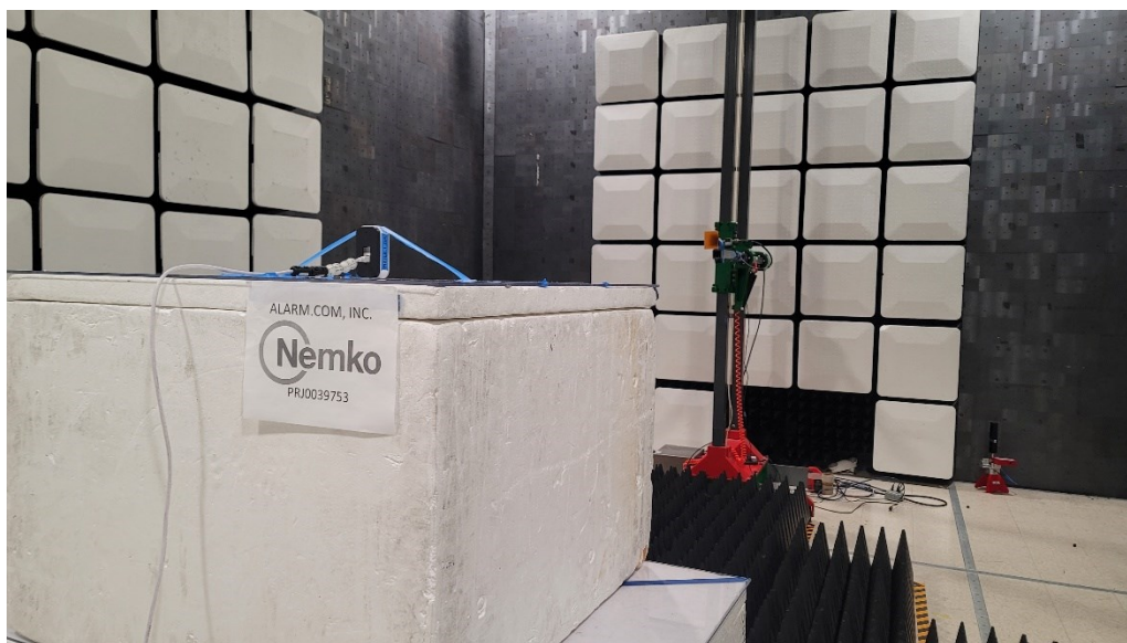
Figure 7 - Radiated emissions above 1 GHz (18 – 26.5 GHz), rear view.
