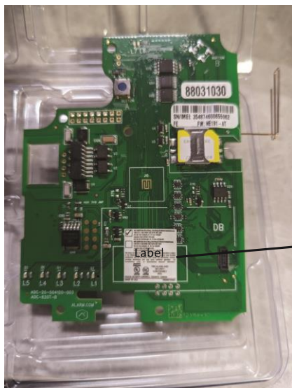
Top of the PCB showing the label location.
