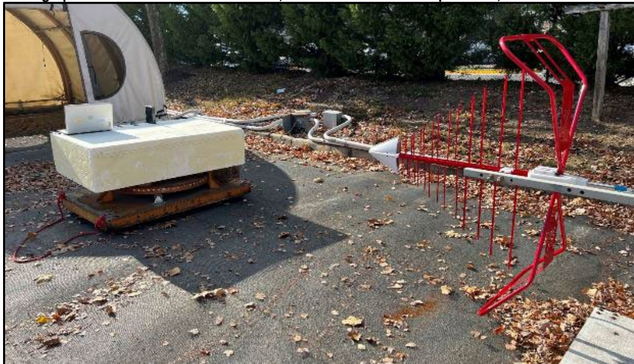
Photograph 7: Radiated Emissions, Unintentional Test Setup <1 GHz, Front View
