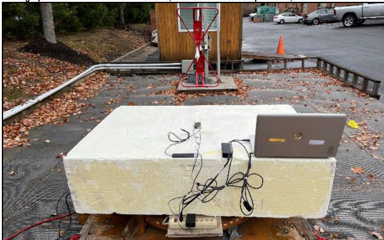
Photograph 4: Radiated Emissions, Intentional Test Setup <1 GHz, Rear View
