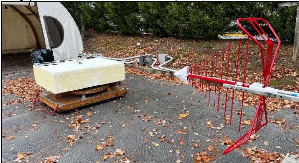
Photograph 4: Radiated Emissions, Intentional Test Setup <1 GHz, Rear View
