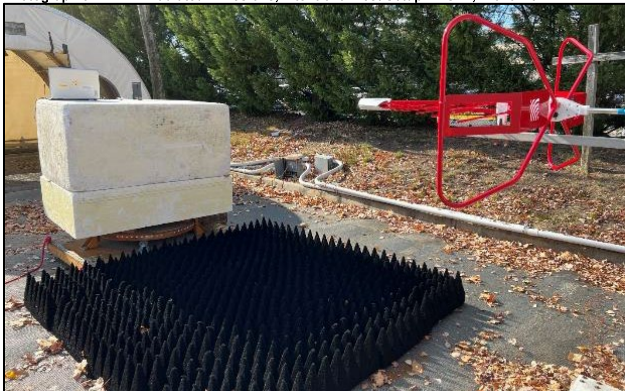
Photograph 6: Radiated Emissions, Intentional Test Setup >1 GHz, Rear View
