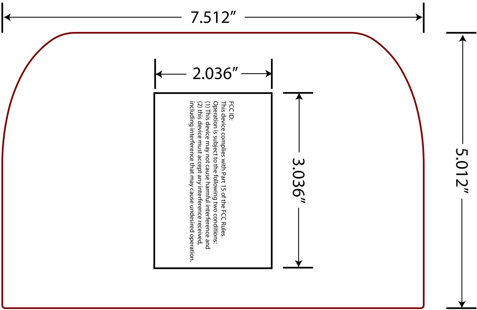
FCC Certification Label will be displayed on the bottom of the unit as pictured. A sticker will be created measuring 3" by 2" and positioned in the recessed area on the bottom of the unit.
