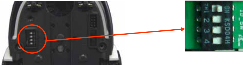
< The location of Robot Speed Control Dip Switch >
