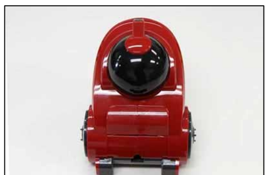
6. The shape after separating a magnetic ball holder from the robot
