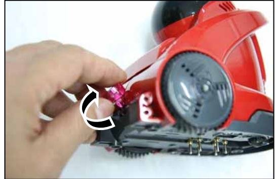
4. Lift the Magnetic ball holder.
