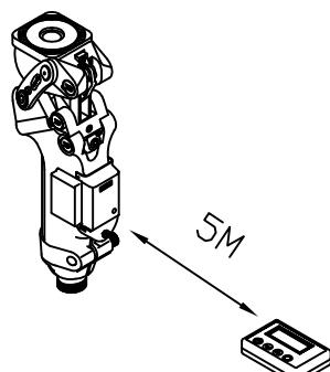
2.3 The effective distance for the remote controller is 3 meters. Make sure there is no obstacle or barrier between the remote controller and knee joint.
