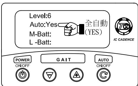
2.2 When the remote controller is setted in the (Yes) auto-position, the IC KNEE JOINT can adjust to the most suitable gait speed for the user.
