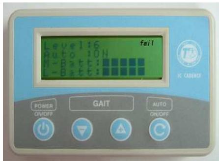
2.2 The remote controller calculates the speed and category level after the first movement of the knee joint. If it is in the "ON" position, the IC will adjust automatically without any further
