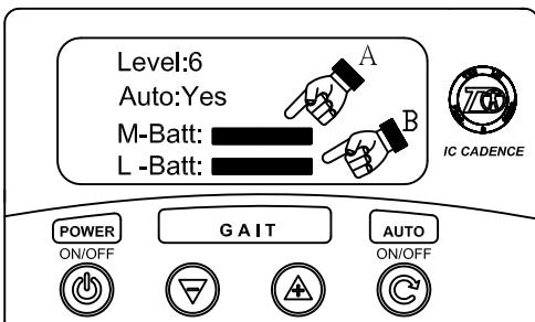
2.4 The power consumption of the battery can be detected by the remote controller when the knee joint is moving.
