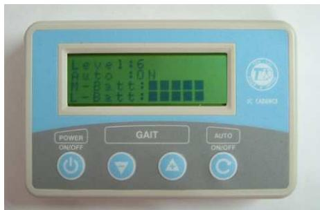
2.4 The power consumption of the battery can be detected by the remote controller when the knee joint is moving.
