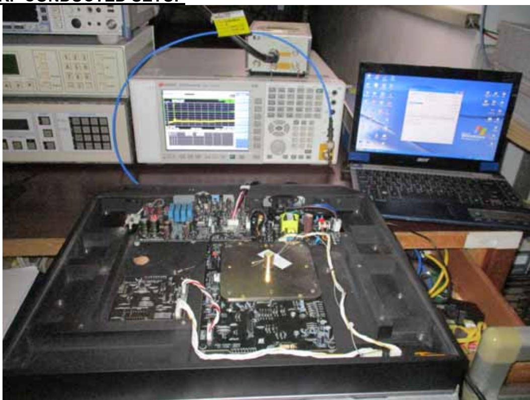
**CONDUCTED EMISSION MEASUREMENT SETUP**
