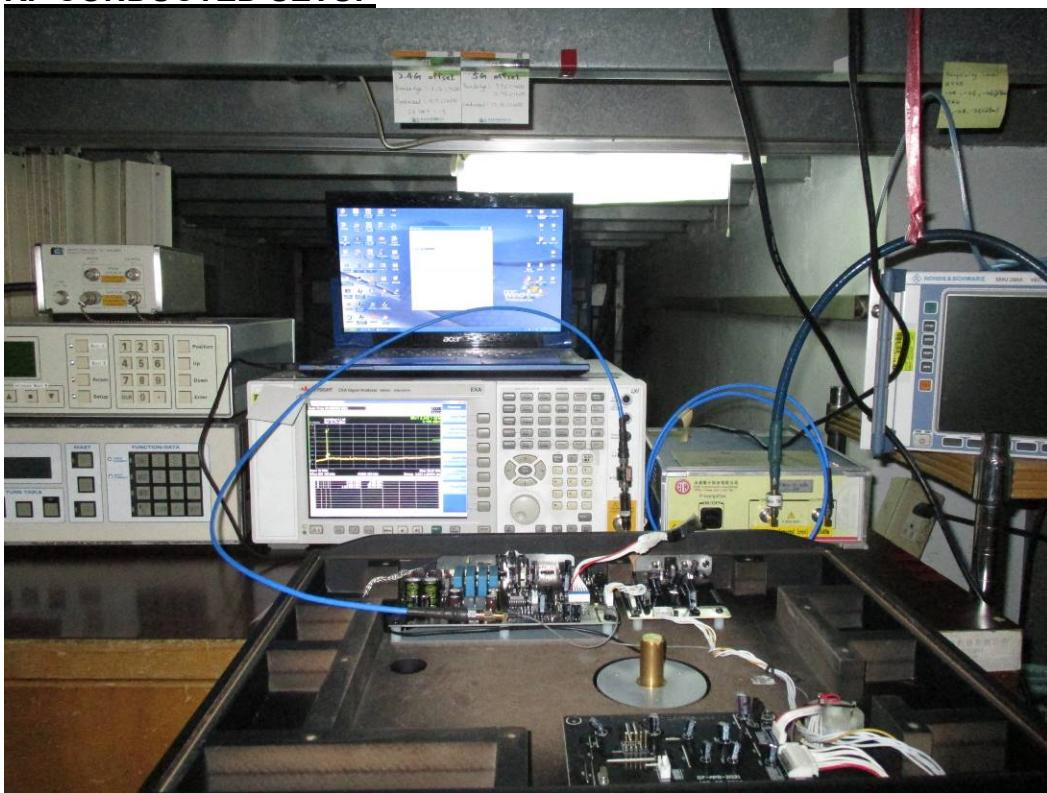
**CONDUCTED EMISSION SUREMENT SETUP****MODE: PHONO DIRCET OFF**
