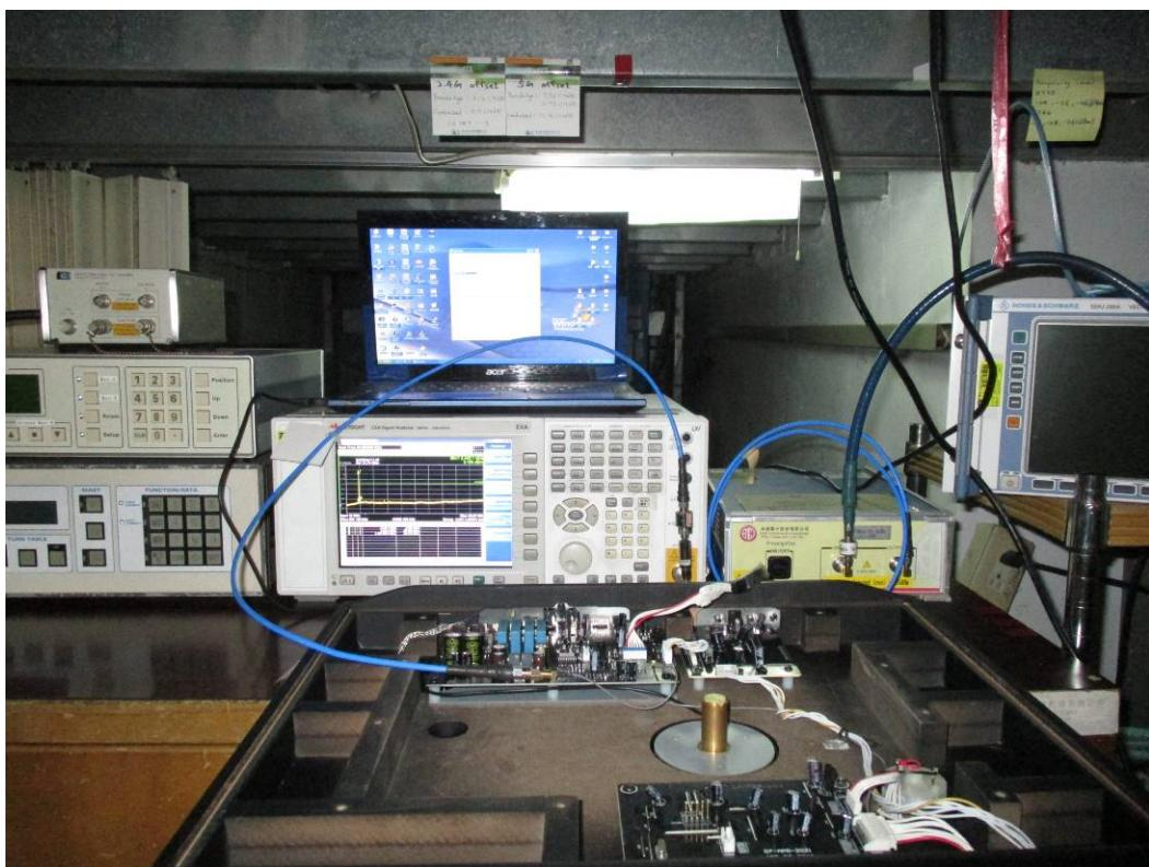
**CONDUCTED EMISSION SUREMENT SETUP****MODE: PHONO DIRCET OFF**
