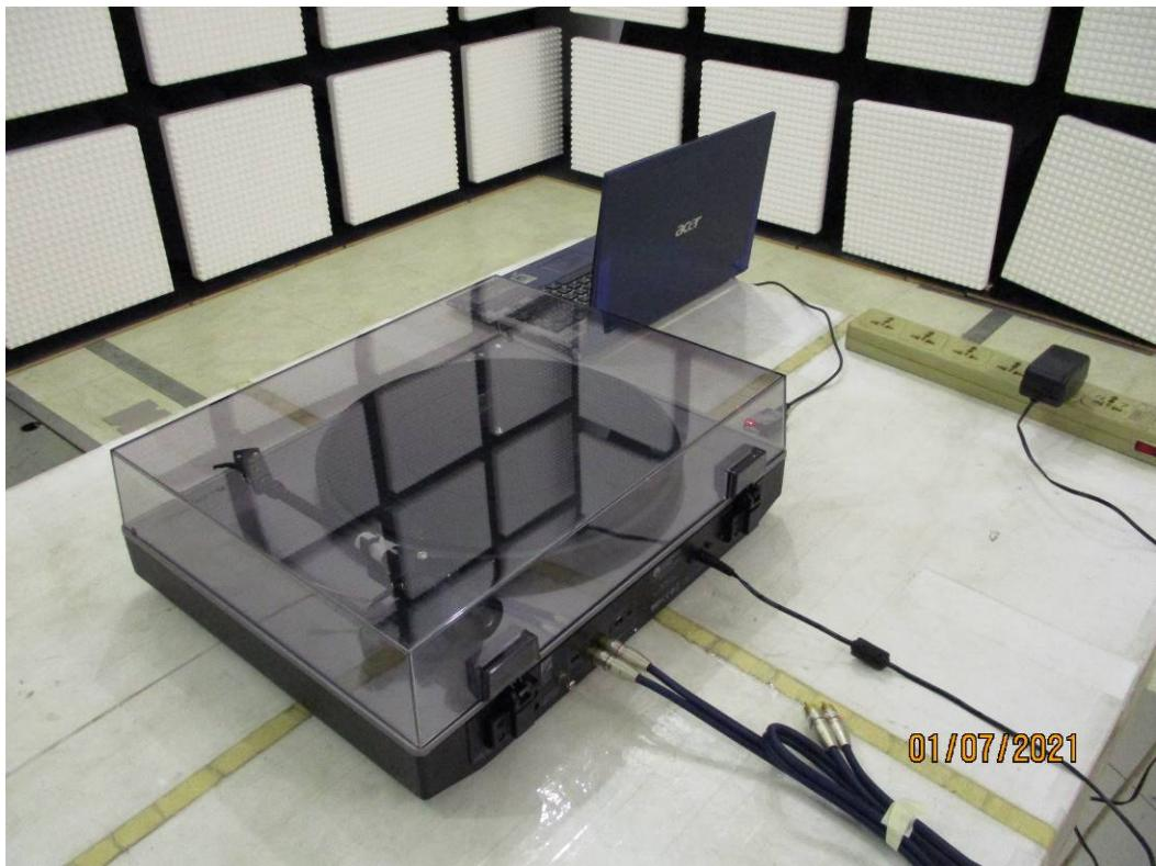
**RADIATED RF MEASUREMENT SETUP****Above 1GHz**
