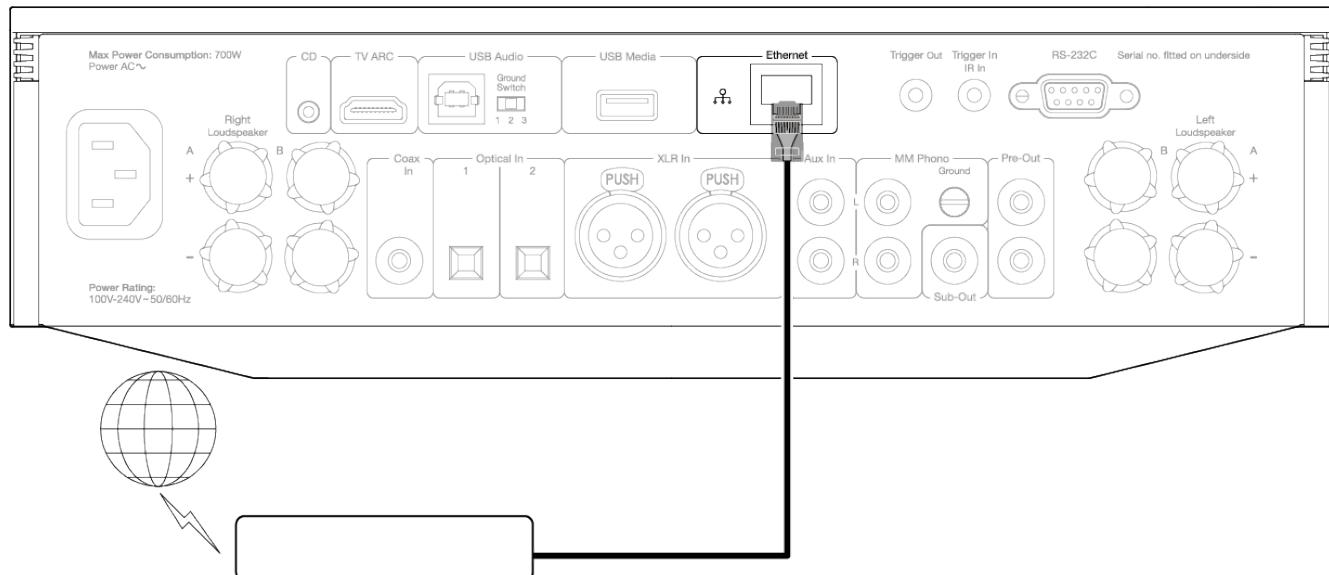
Connect a network cable between the Evo and your router.
