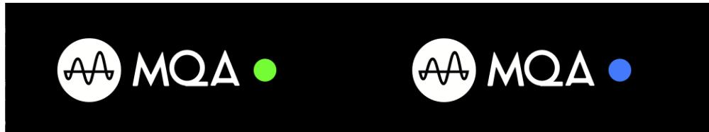
The front panel will display MQA green or blue to indicate that the unit is decoding and playing an MQA stream or file, and denotes provenance to ensure that the sound is identical to that of the source material. It displays MQA blue to indicate it is playing an MQA Studio file, which has either been approved in the studio by the artist/producer or has been verified by the copyright owner.
