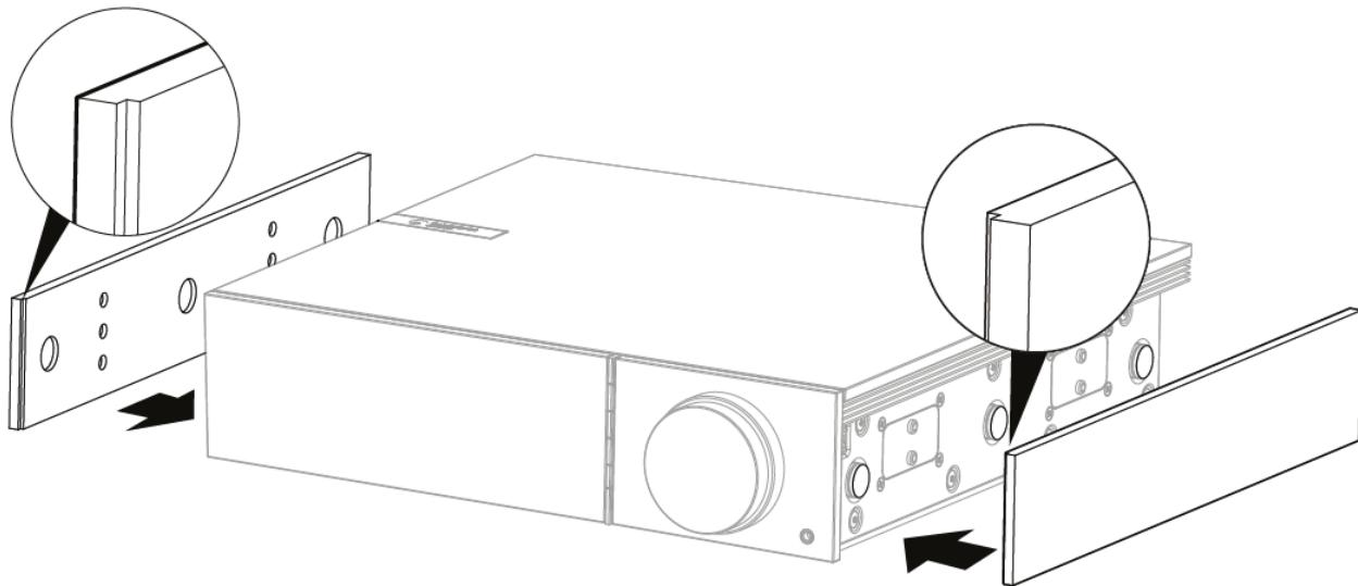
When installing new magnetic side panels, please ensure that the groove cuts are aligned with the direction of the front panel. Insert from the rear by holding the rear of the panel.
