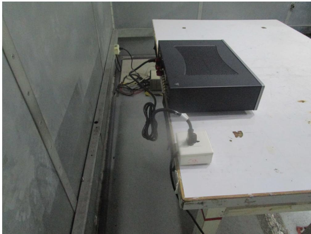
**Radiated Emissions Test Photos****9 kHz to 30 MHz**
