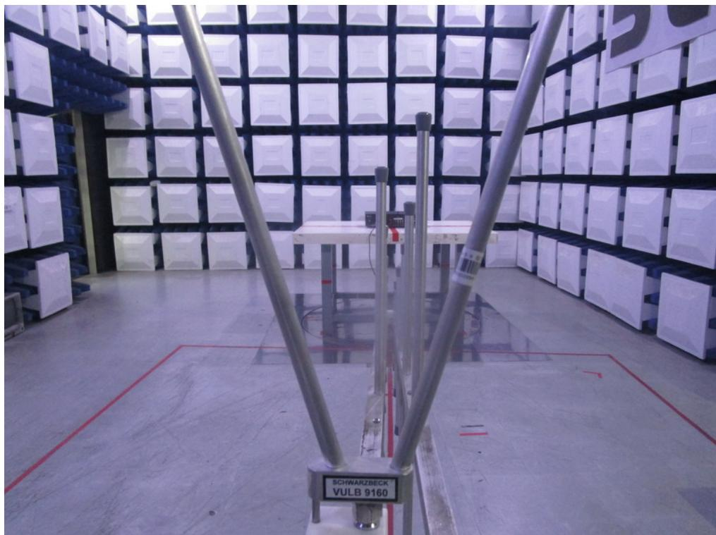
**Radiated Emissions Test Photos****1 GHz to 18 GHz**
