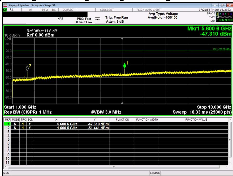
**RE\_1 - 10 GHz\_Server to Donor\_451.5 MHz\_B5 connected\_1 - 10 GHz HP filter for B5**
