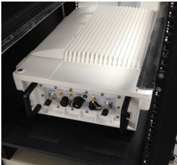
Figure 7: Edge Repeater rack mounted on a vented flat tray.
