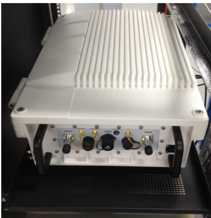
Figure 8: Raised end Edge Repeater rack mounted on a vented flat tray.
