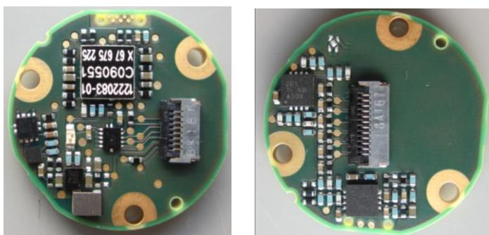
On the evaluation board there is a  $\mu$ -controller that generates its own clock. This internal system clock is 24 MHz. This tact is not given to the outside world. The FRAM is connected to the  $\mu$ -controller via SPI (6MHz).
