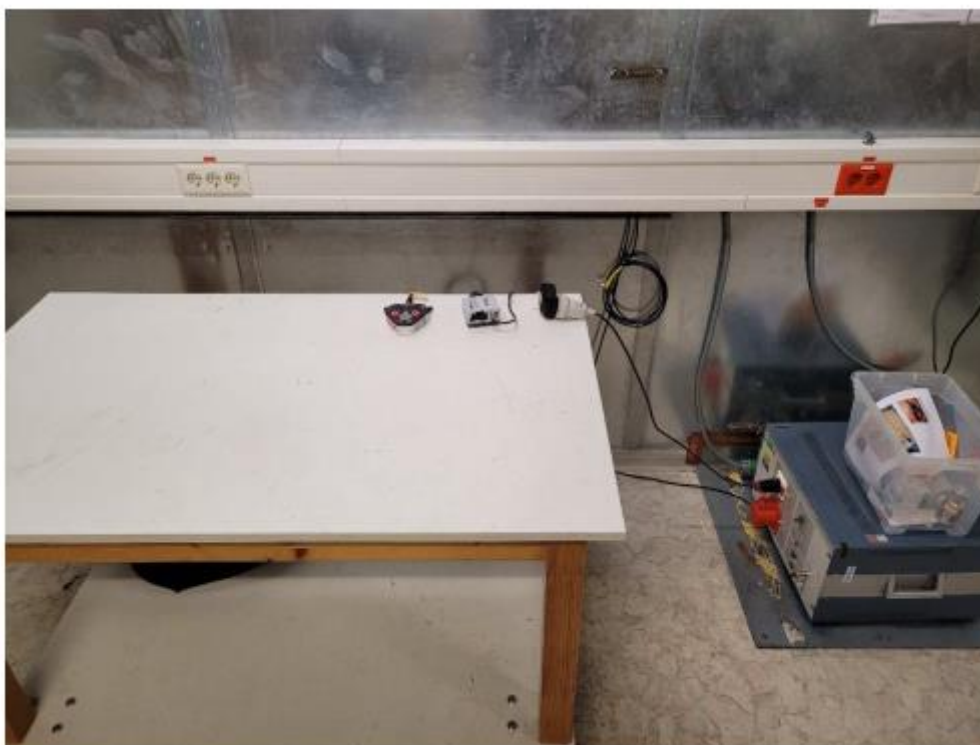
AC Powerline Conducted
