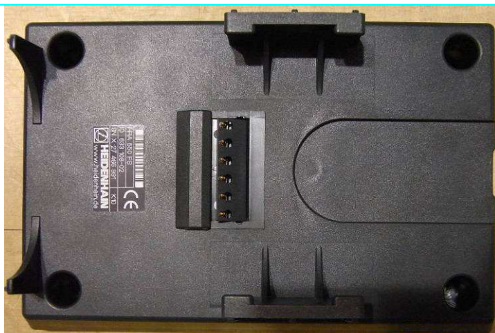
External view of interface between controllers and CNC machine for recharging and wireless communication with the portable controller
