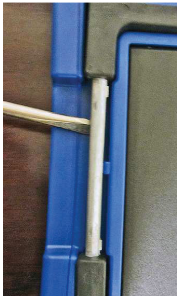
Figure 1-8. Screwdriver inserted beneath stand crossbar
