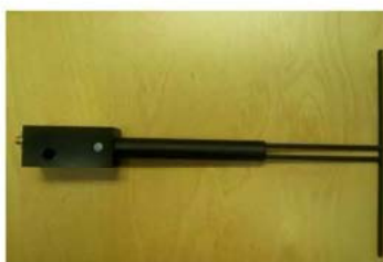
Figure 1 – MVG COMOSAR Validation Dipole
