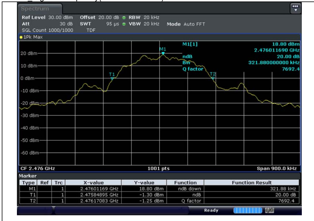
GFSK_Highest Frequency(20 dB Bandwidth)
