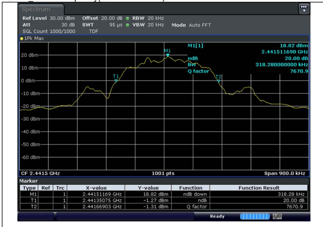
GFSK_Middle Frequency(20 dB Bandwidth)
