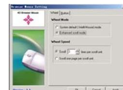
as this picture show, the upside is for setting mode of scroll wheel, the underside is for setting speed of scroll wheel
