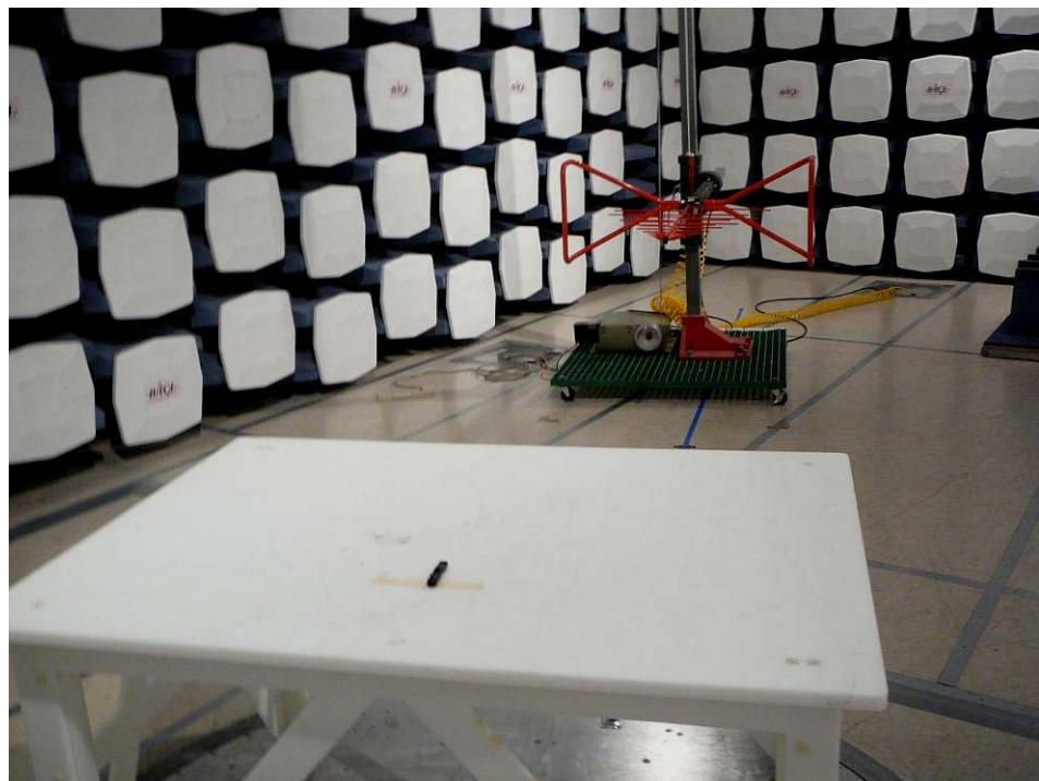
**14.5 Radiated Emission above 1 GHz Front View at 3 Meter**
