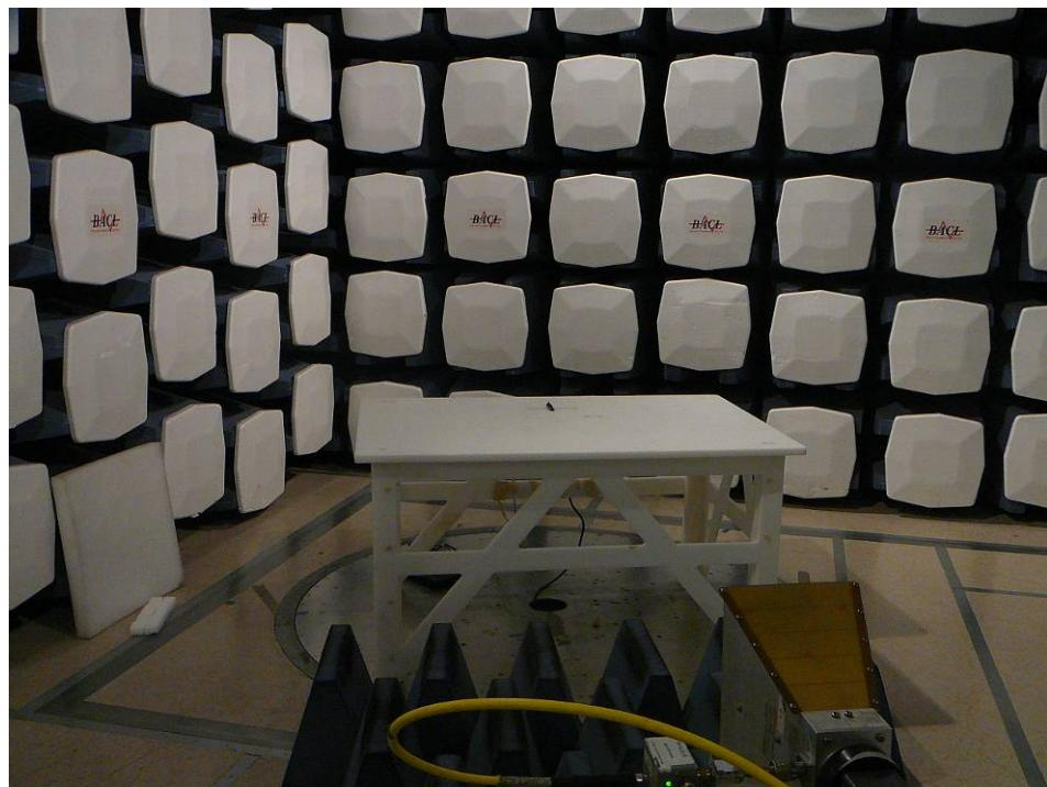
**14.6 Radiated Emission above 1 GHz Rear View at 3 Meter**
