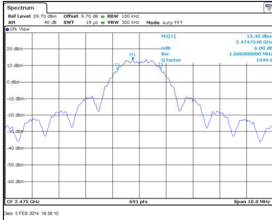
Figure 7.3.2-3: 6dB Bandwidth Plot – 2480 MHz
