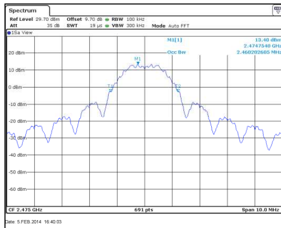
Figure 7.3.2-6: 99% Bandwidth Plot – 2480 MHz
