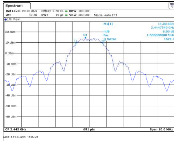
Figure 7.3.2-2: 6dB Bandwidth Plot – 2440 MHz
