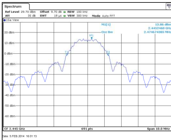
Figure 7.3.2-5: 99% Bandwidth Plot – 2440 MHz
