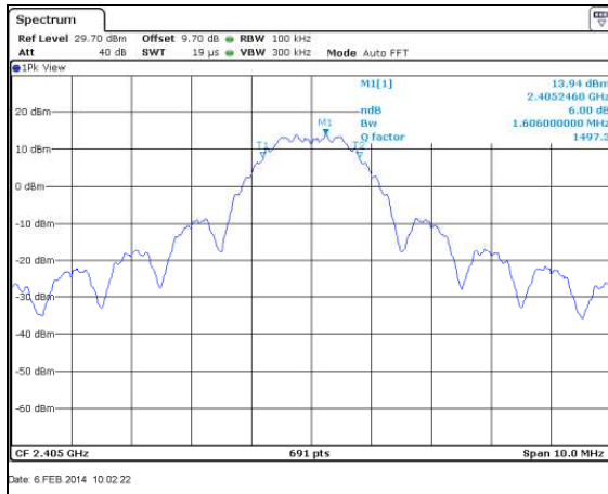
Figure 7.3.2-1: 6dB Bandwidth Plot – 2405 MHz
