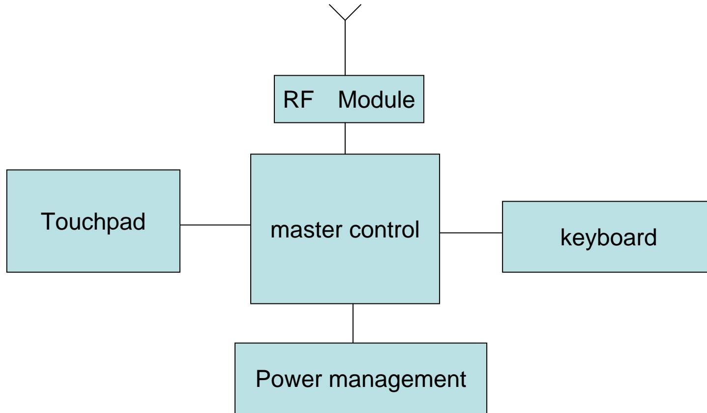
Loop description: The Master Control reads the data from Keyboard, and collects signals from the Touchpad, then launch out the data by RF Module.
