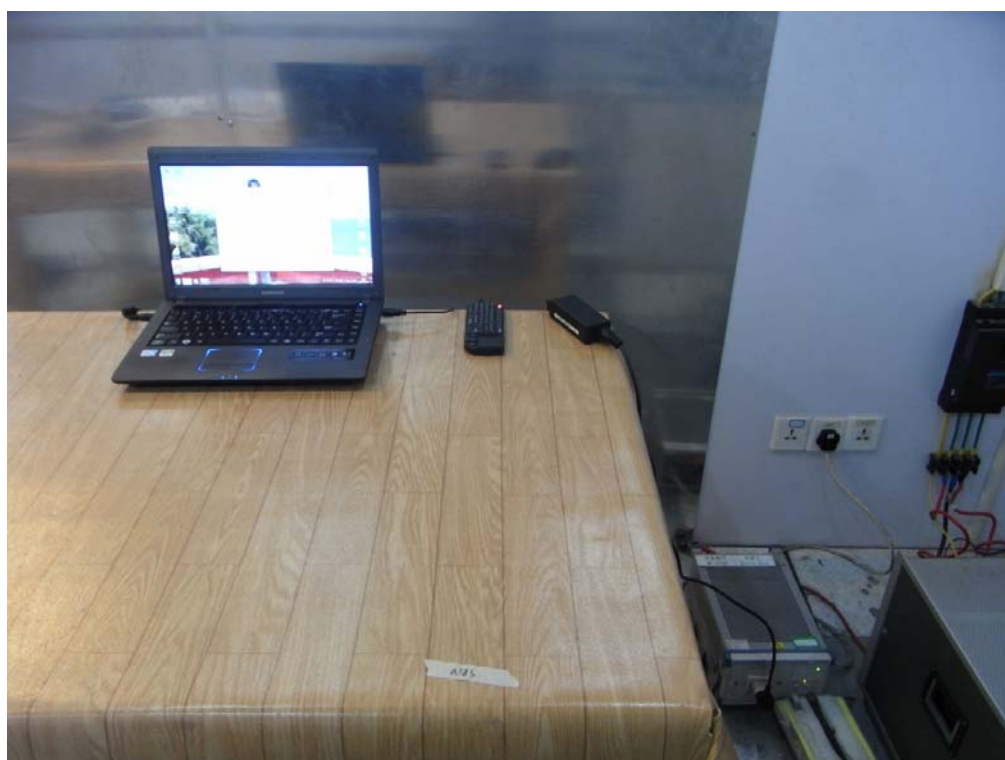
Conducted Emission Test Setup
