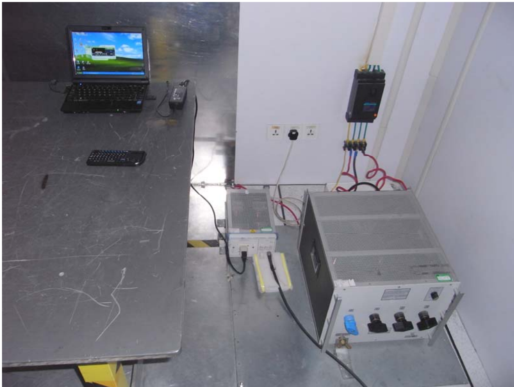
Line Conducted Emission Test Setup
