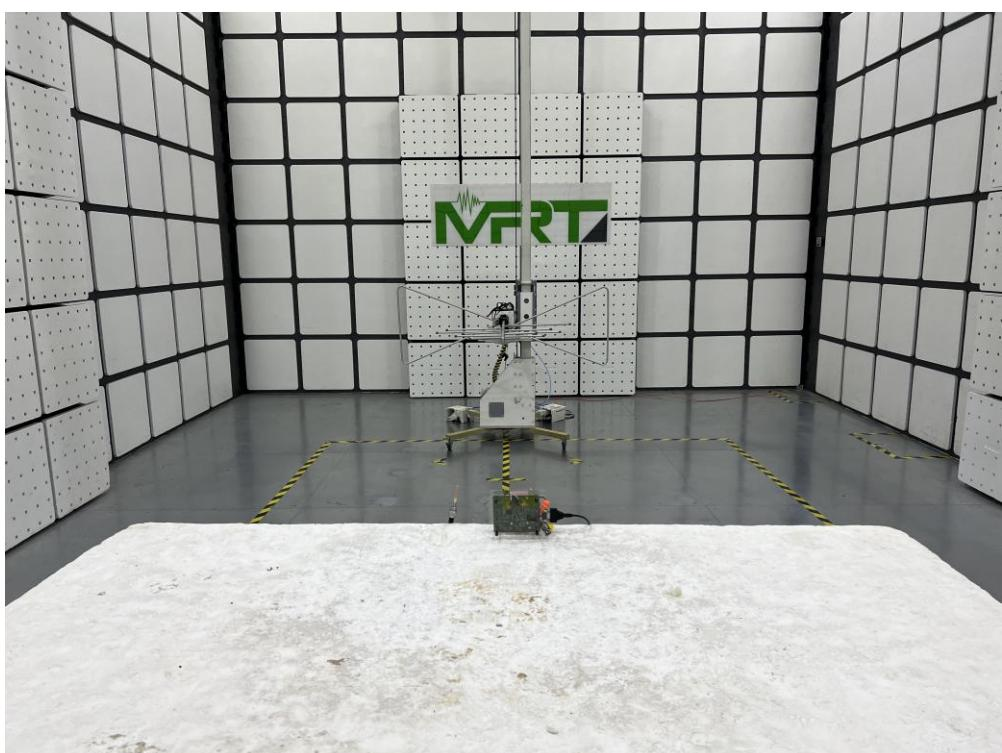
Description: Radiated Emissions Test Setup for 960MHz ~ 18GHz
