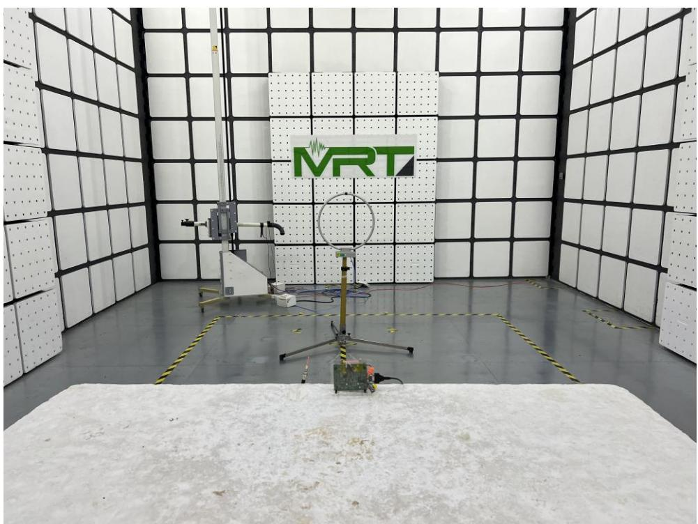
Description: Radiated Emissions Test Setup for 30MHz ~ 960MHz
