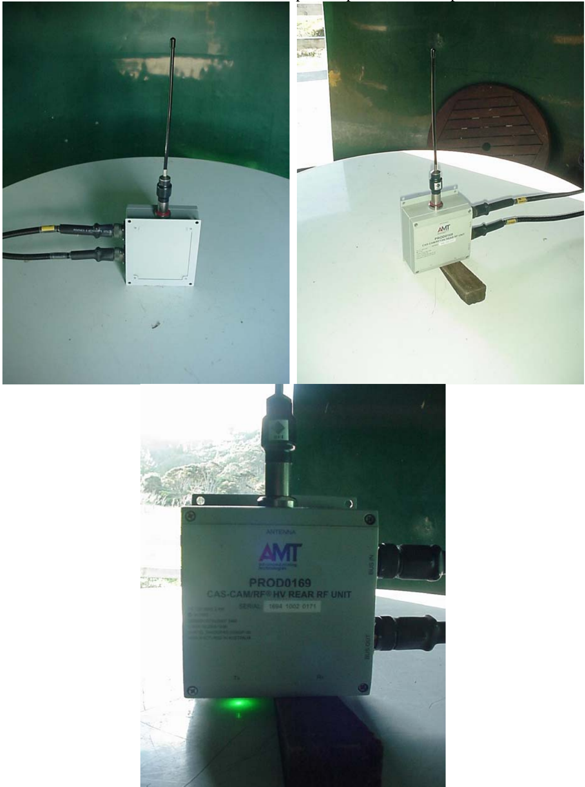
Radiated emissions test set up – Whip antenna on output
