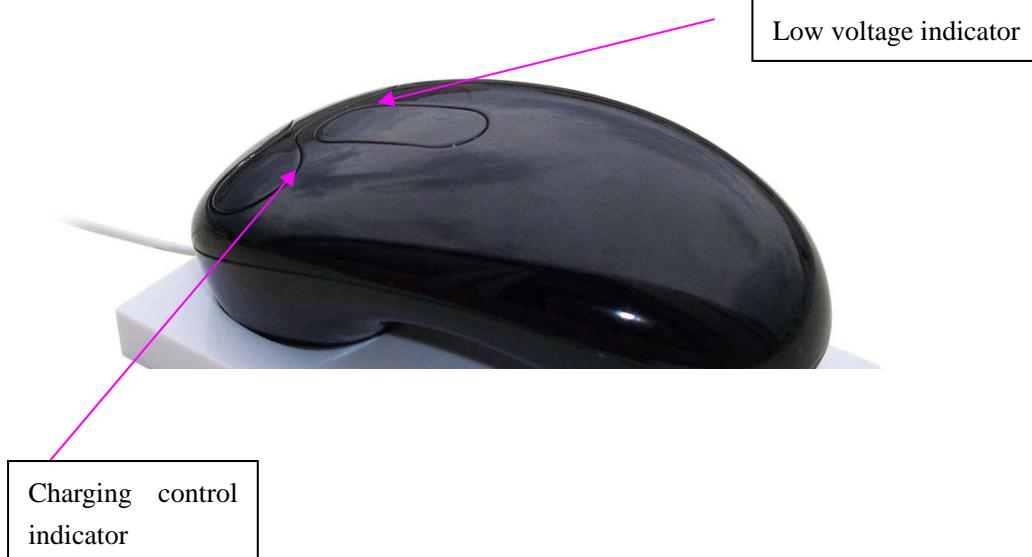
5. Capacitive touch technology to replace the traditional mechanical wheel , when you surf the internet , browse the web , or scrolling the long documents, enlarge the photo you just need use a finger slide the touch area easily . When finger slide up, it will move up the scroll wheel or enlarge the image . When finger slide down , it will move down the scroll or narrow the image
