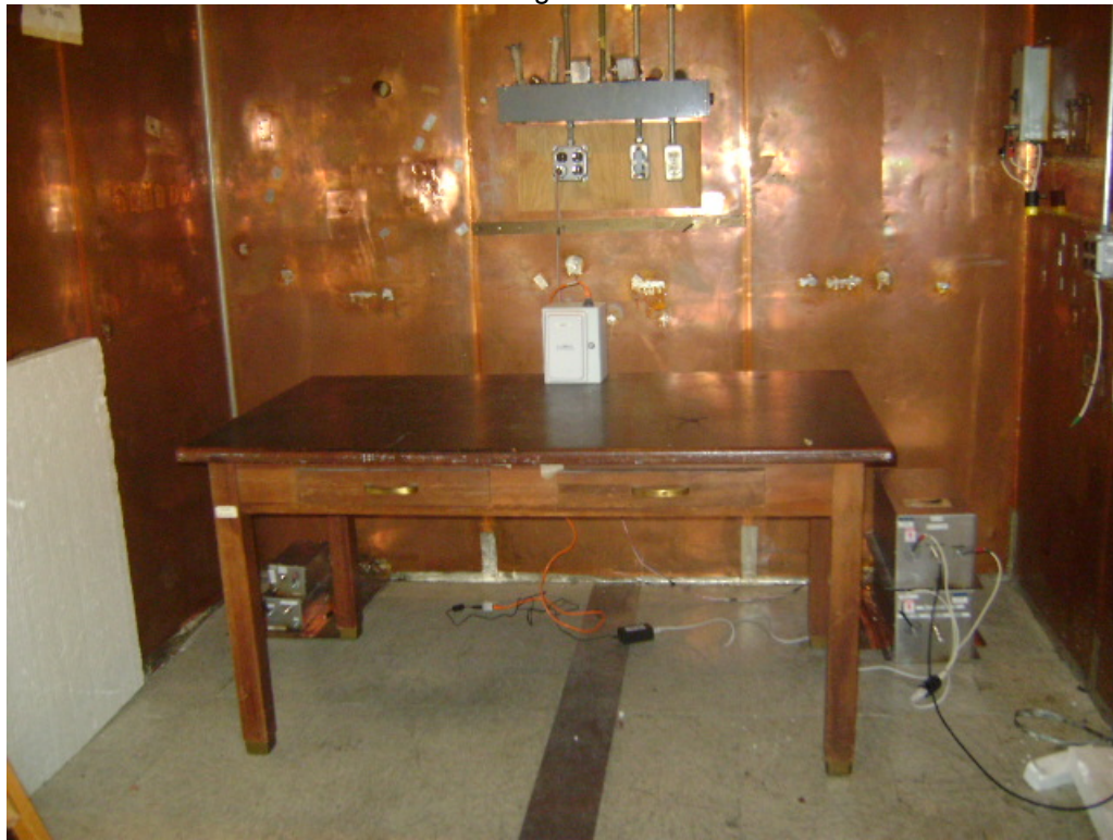
Test Setup for Conducted Emissions
