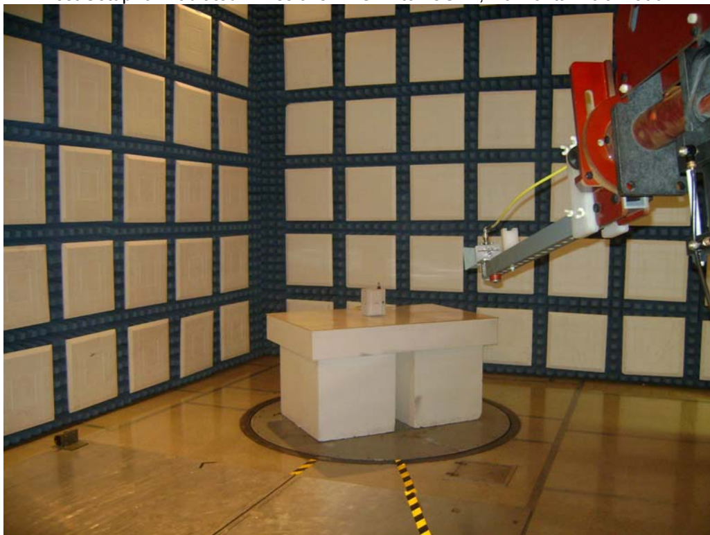
Test Setup for Radiated Emissions – 2GHz to 18GHz, Vertical Polarization
