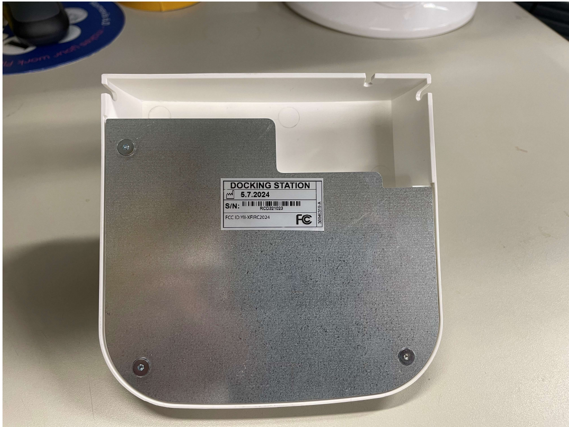
4. Docking station bottom, with LABEL location
