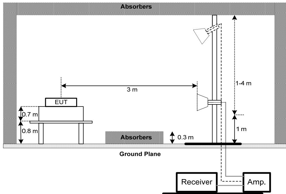
(C) For radiated emissions below 30MHz
