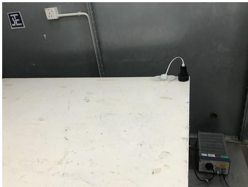
Measurement of Conducted Emission Test Set Up
