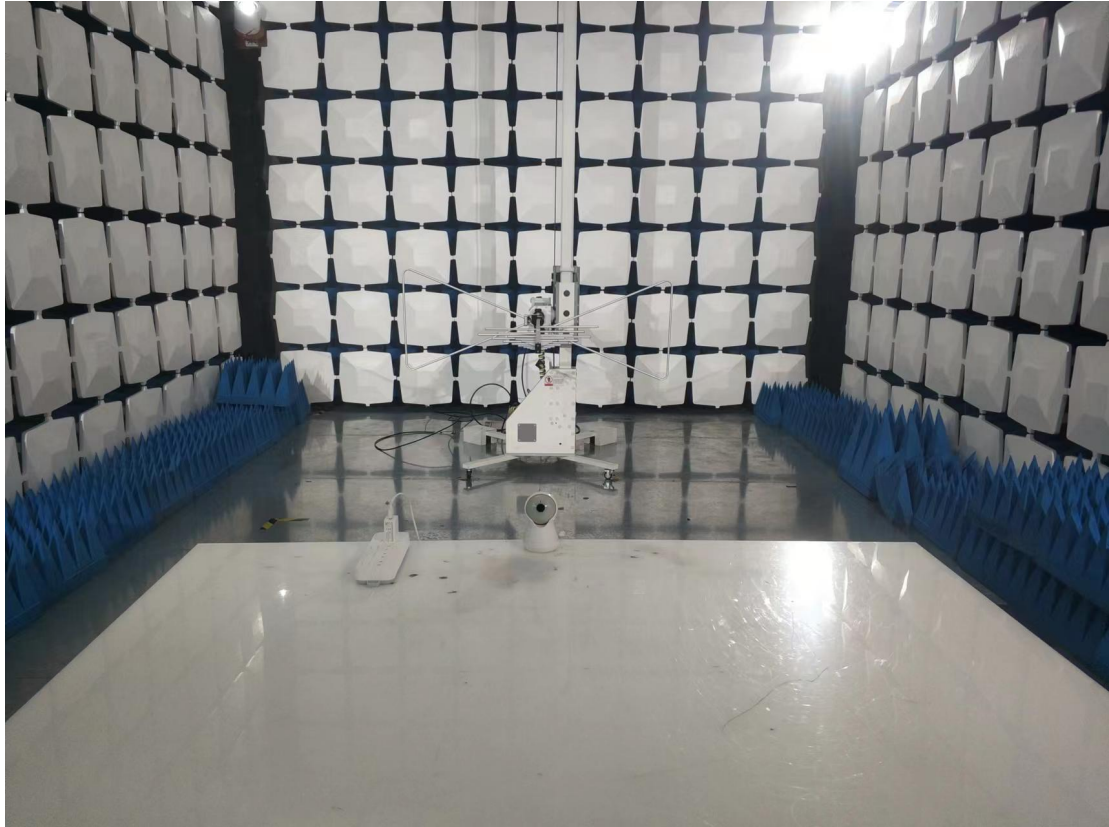
Below 1GHz for radiated emission test setup
