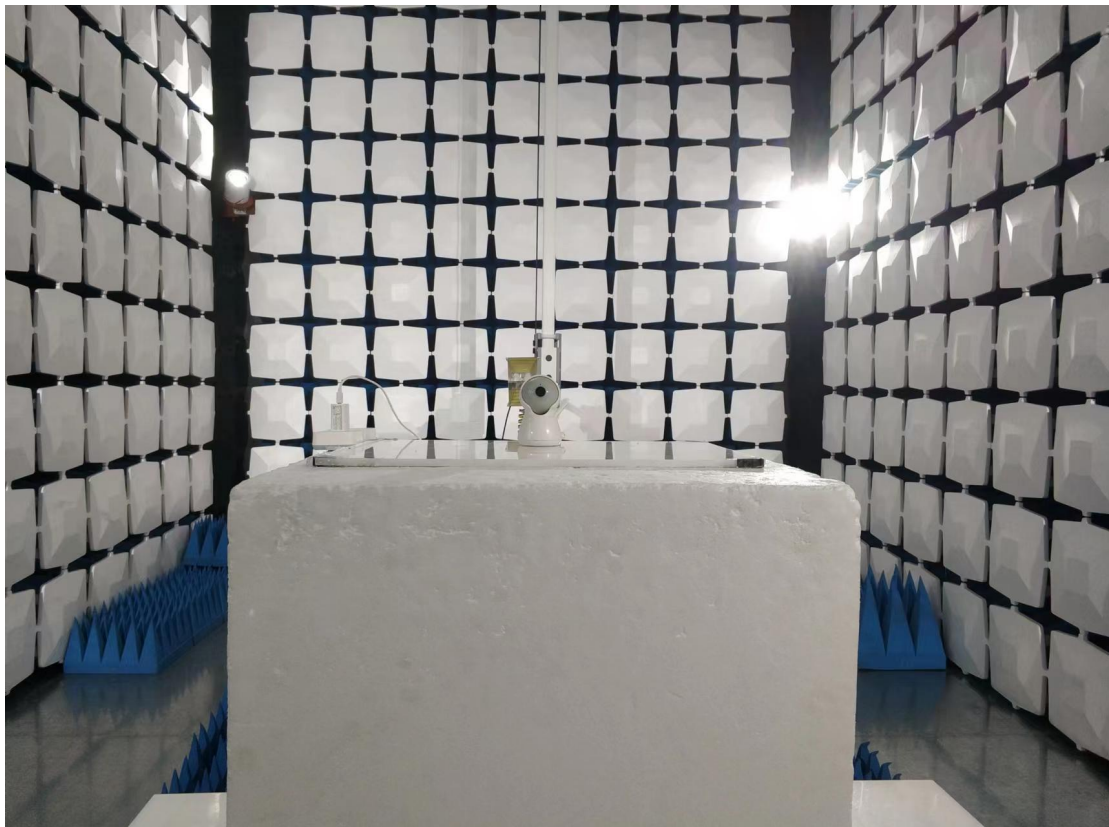
Above 1GHz for radiated emission test setup
