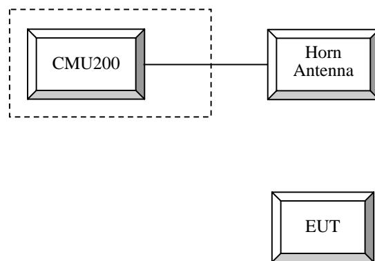
**Block Diagram of Test Setup**
