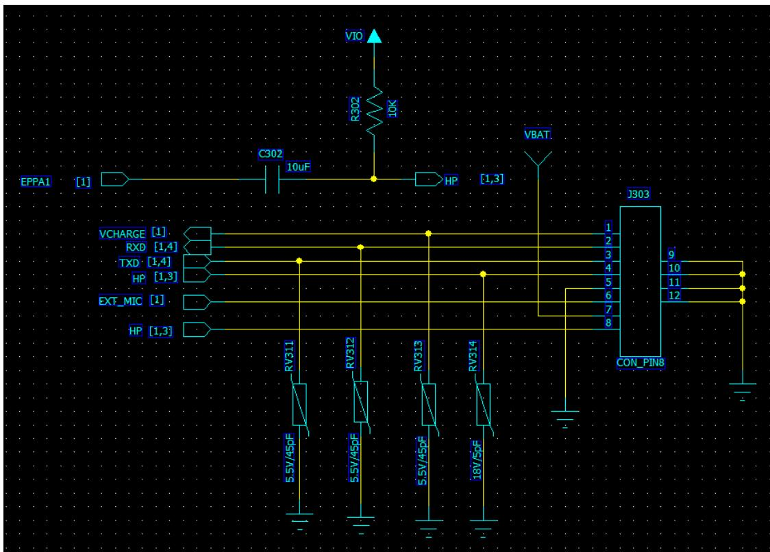
The I/O circuit contains earphone port, UART port, charge input. HP is detecting pin for earphone insert. For normal it is high, and become low when earphone insert.
