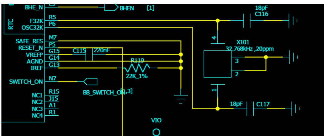
After inserting the battery, VRTC output voltage of 2V, and then the 32.768KHZ crystal start to work. Now press the power on/off switch SW313, then the inner program start initializing. Press the power on/off switch about 2s at normal work status, CPU PMB7880 will detect the signal and start the power off program.
