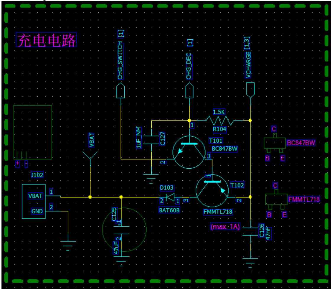
The PMB7880 integrate the charger control circuit. When inserting the charging Adapter, CHG\_DEC detect high level, and start the charging program.
