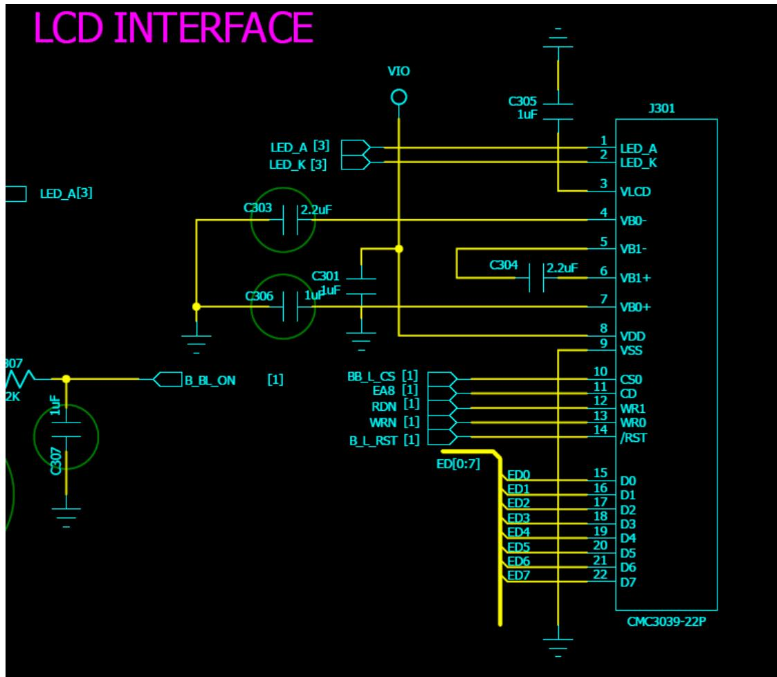
The LCD connects to PMB7880 through FPC. The signals are defined as follows:
