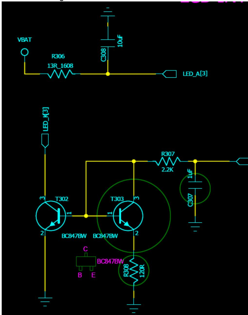
LCD backlight is Control by T302 and T303. B\_BL\_ON enable LCD backlight LED.
