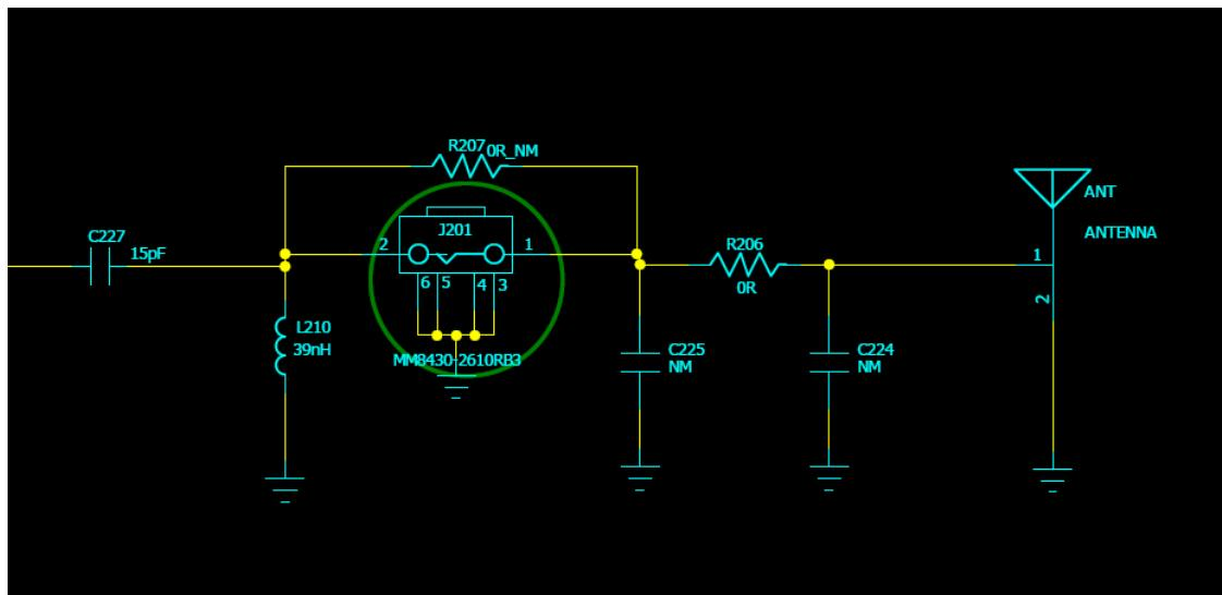
This circuit shows the transmitter and receiver path of GSM/DCS/PCS. The RF signal which is amplified by RF PA transmits to antenna through antenna switch and then eradiate to the air. R206, C224, C225 make up of the antenna matching circuit. When receiver, the antenna receive the RF signal, and then demodulated by PMB7880 after band filter.
