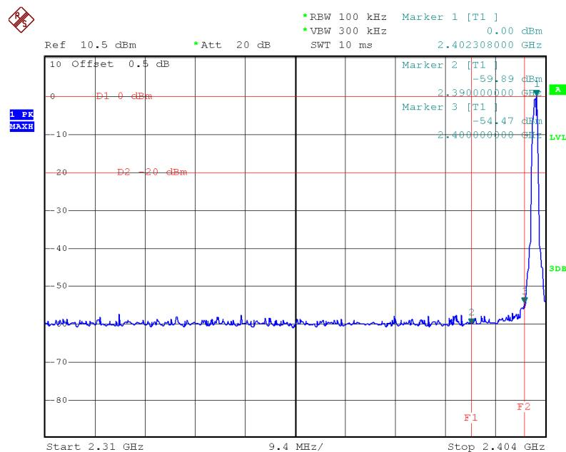
**$\pi/4$ -DQPSK - Band Edge: Right Side**
