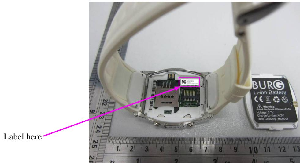
The label shown shall be permanently affixed at a conspicuous location on the device and be readily visible to the user at the time purchase (Labeling requirements per 2.925)
